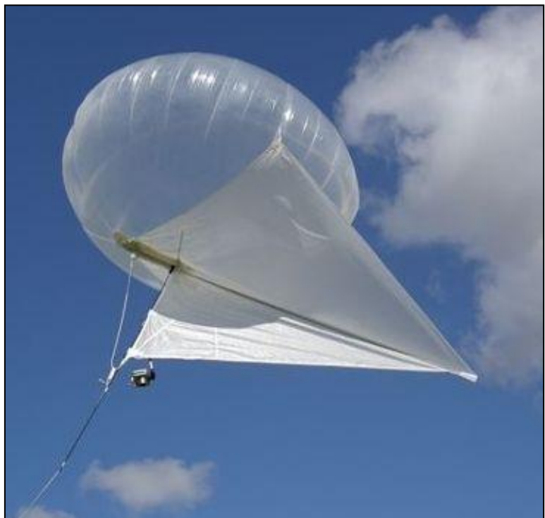
Figure 8: Allsop Helikite deployed with a high resolution surveillance camera suspended below the balloon. Photo credit Allsop Helikites
